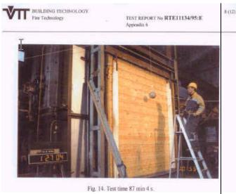
one test during 90-minutes the requirements of loadbearing and separating wall constructions presented in the standard DIN 4102 Part 2 Edition 1977."
